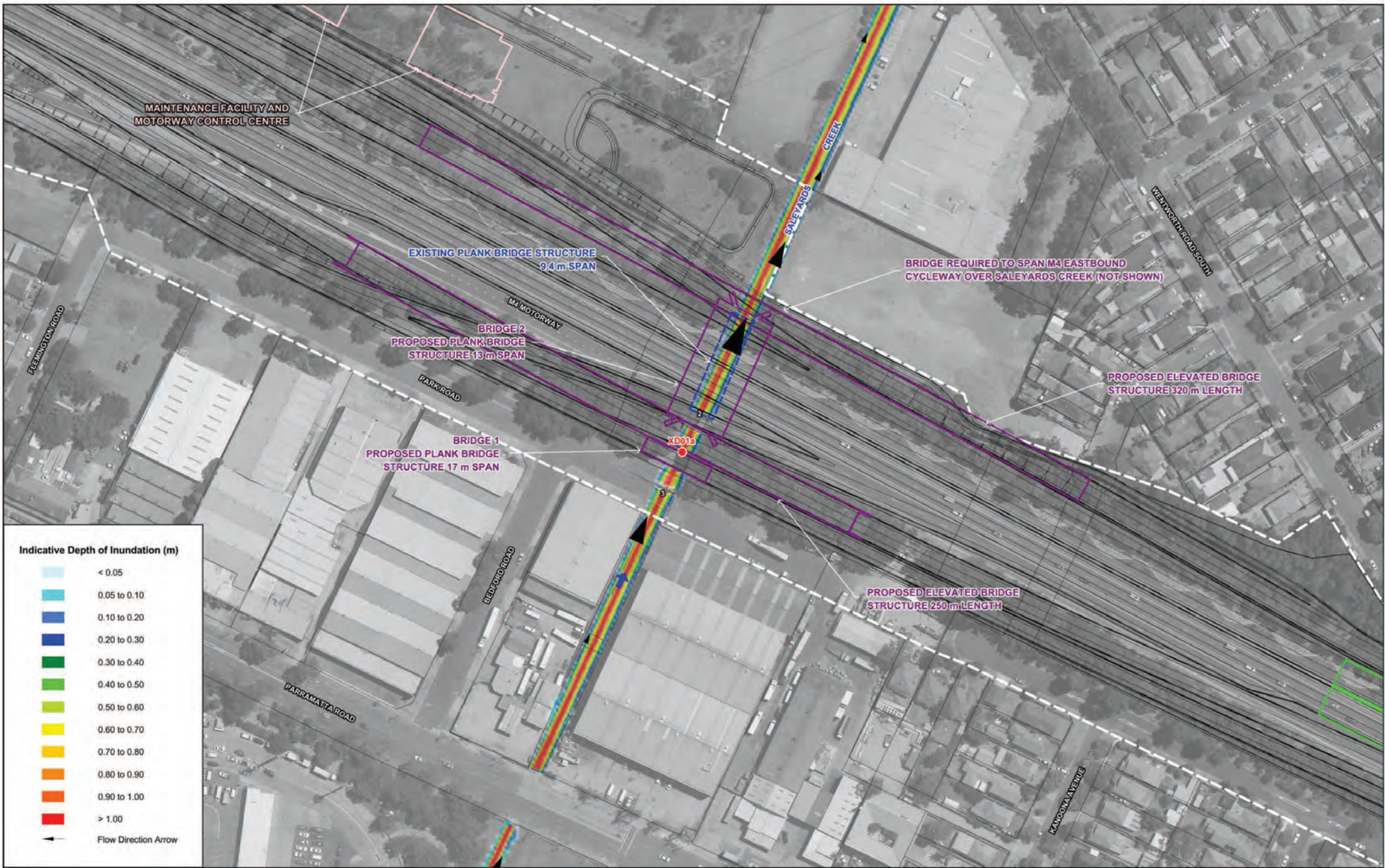
WESTCONNEX M4 EAST EIS SURFACE WATER: FLOODING AND DRAINAGE Figure D1 POST-CONSTRUCTION FLOODING PATTERNS M4 MOTORWAY (SALEYARDS CREEK) 5 YEAR ARI
