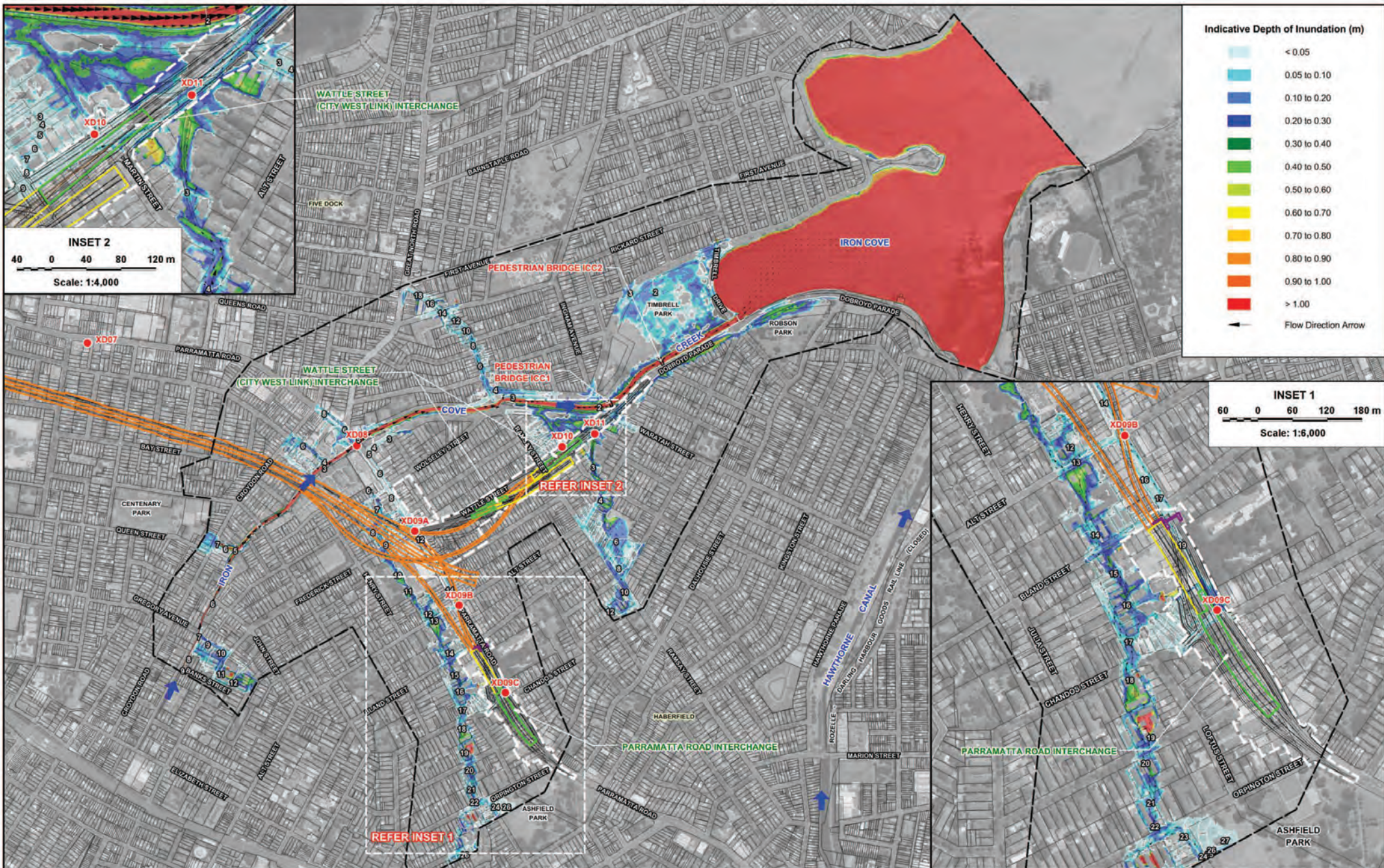
WESTCONNEX M4 EAST EIS SURFACE WATER: FLOODING AND DRAINAGE Figure C14 DOBROYD CANAL (IRON COVE CREEK) TUFLOW MODEL RESULTS 5 YEAR ARI PRESENT DAY CONDITIONS
