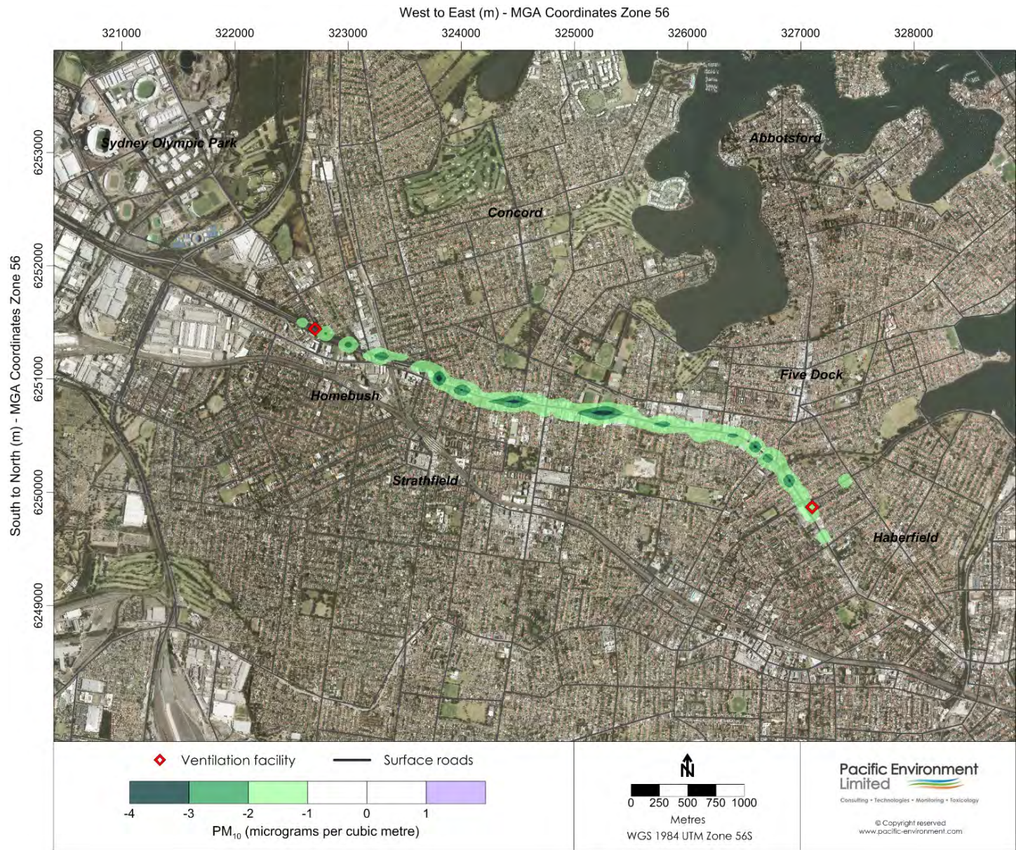
Figure 8-55 Contour plot showing change in annual mean PM 10 with the project (2021-DS)
