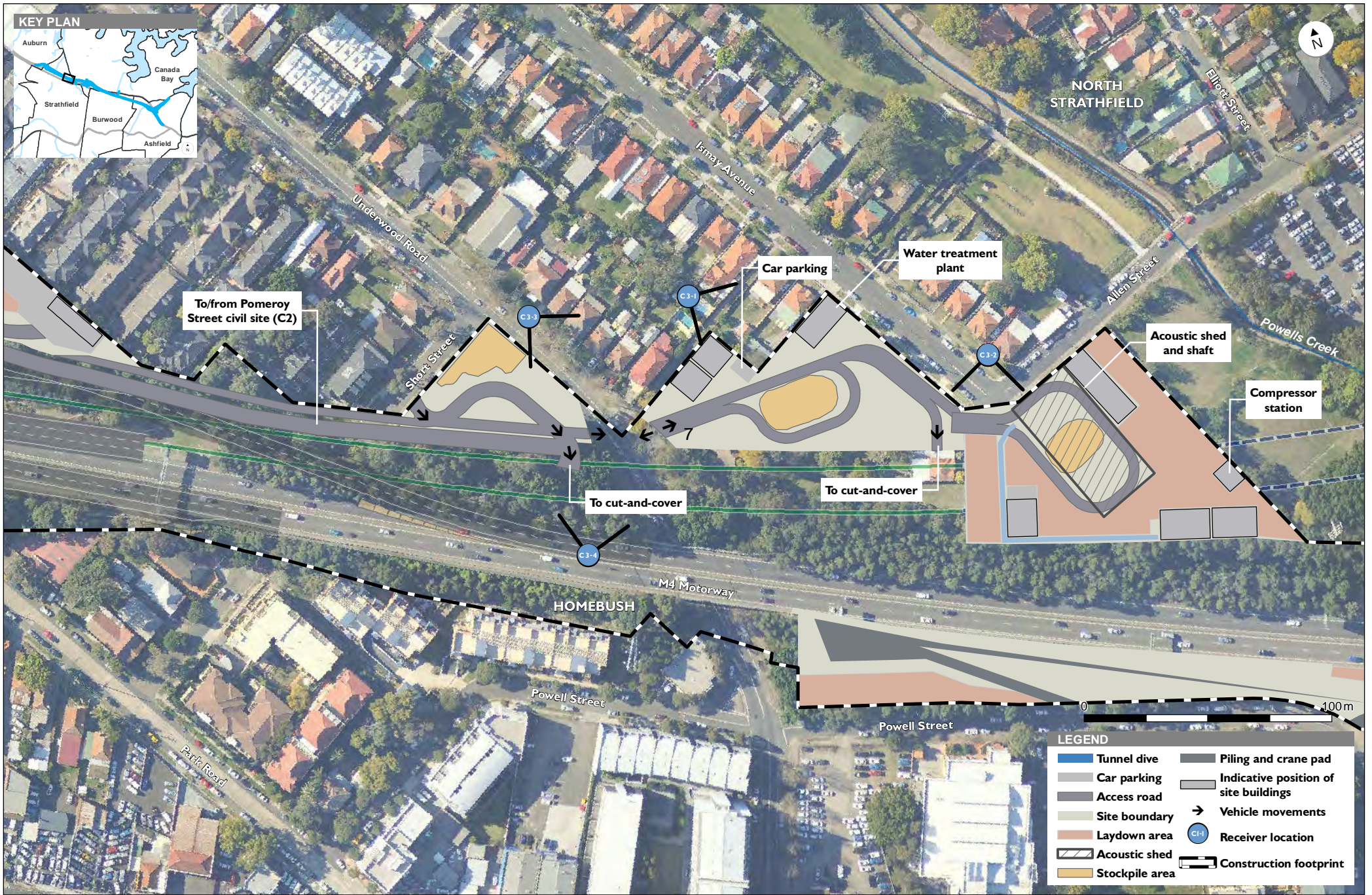
Figure 13.7 Underwood Road civil and tunnel site (C3) receivers
