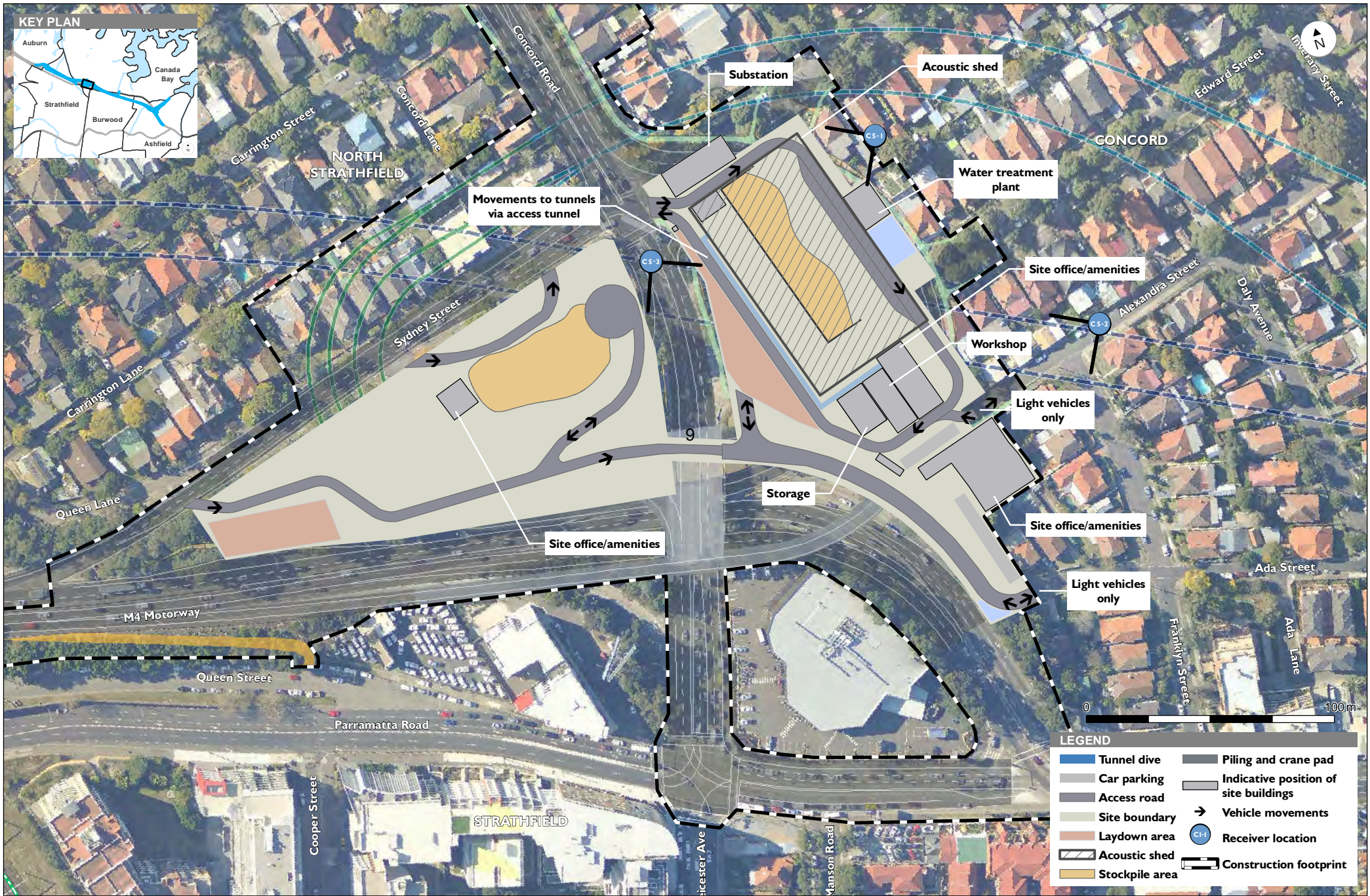
Figure 13.9 Concord Road civil and tunnel site (C5) receivers
