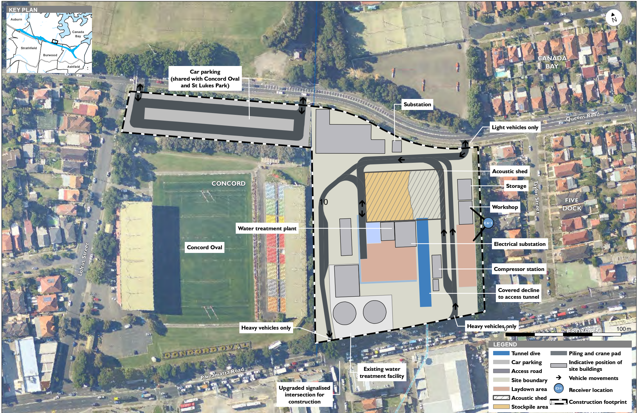
Figure 13.10 Cintra Park tunnel site (C6) receivers
