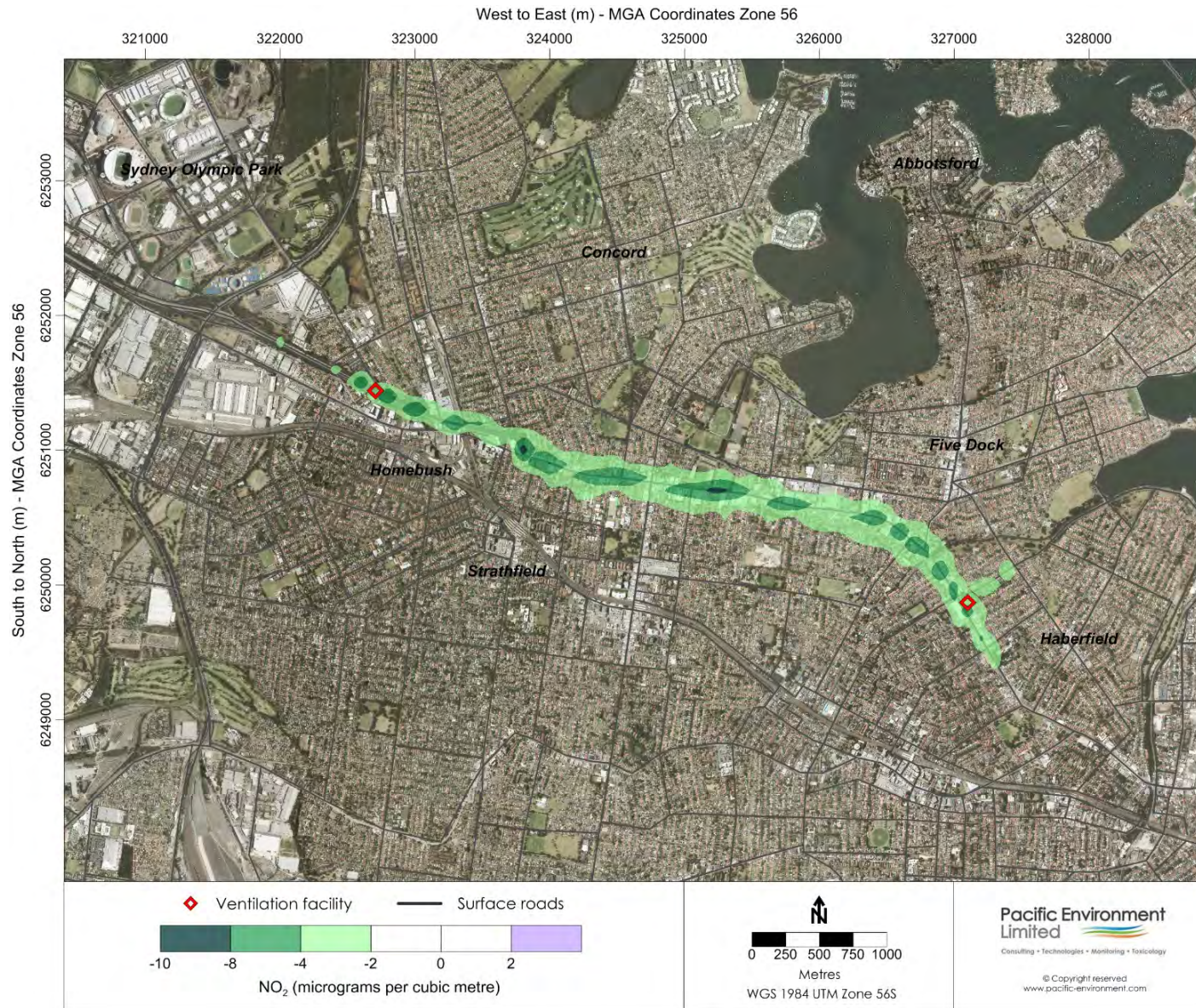
Figure 9.32 Contour plot showing change in annual mean NO 2 with the project in 2021 (2021-DS)
