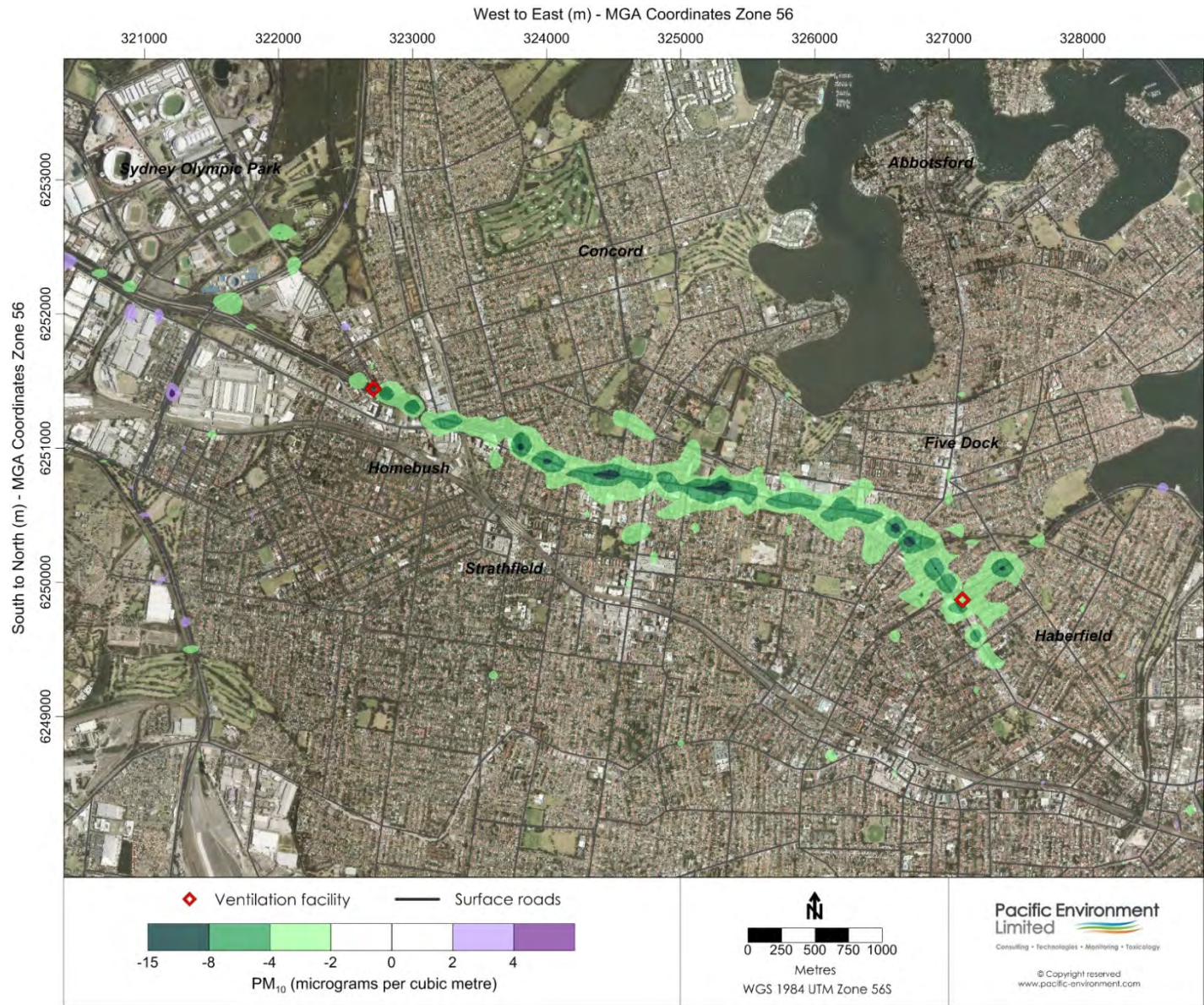
Figure 9.48 Contour plot showing change in maximum 24-hour PM 10 with the project (2021-DS)
