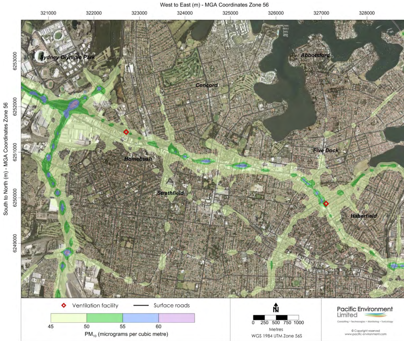
Figure 9.46 Contour plot showing maximum 24-hour average PM10 without the project in 2021(2021-DM)
