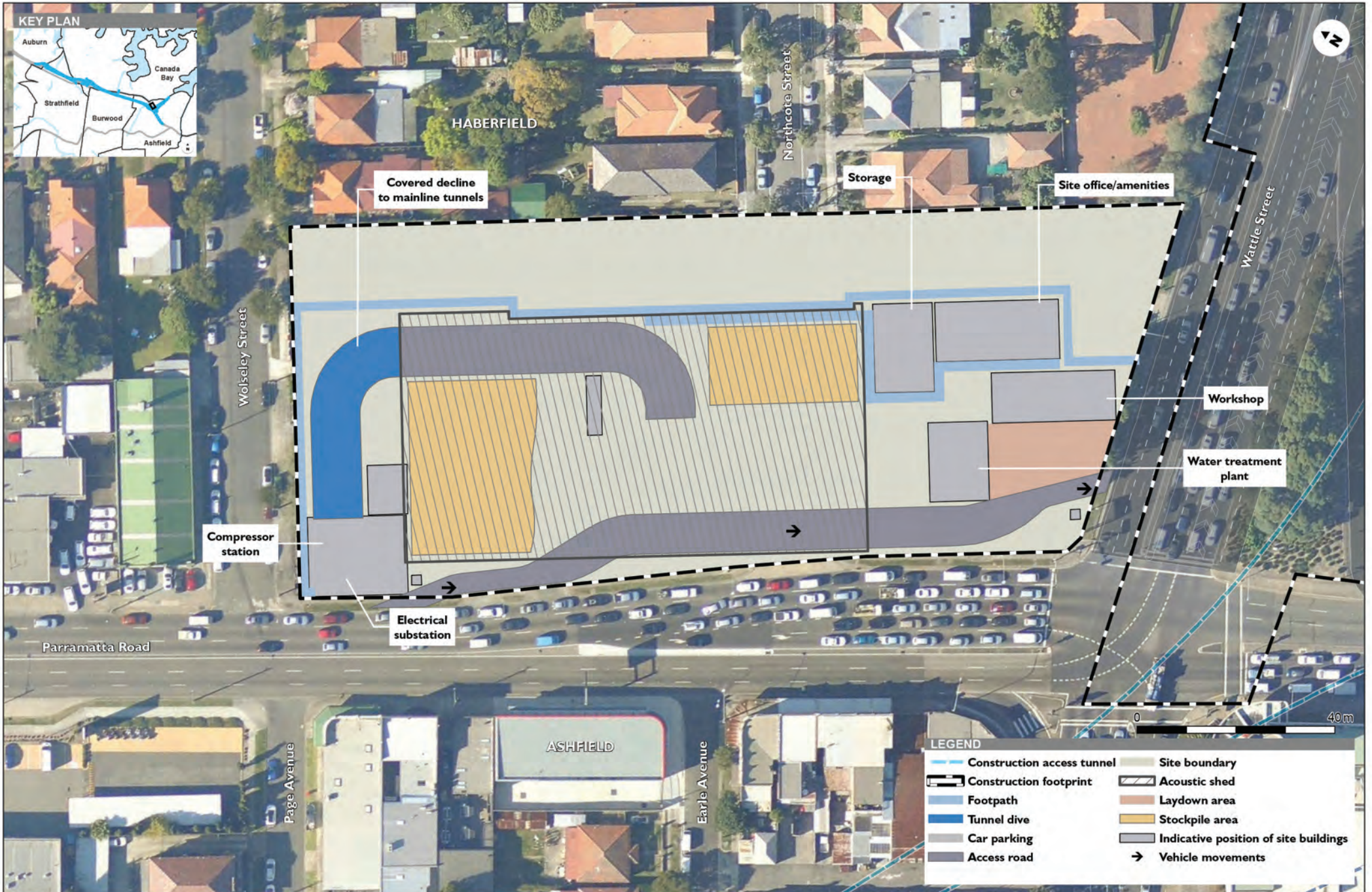
Figure 6.15 Indicative Northcote Street tunnel site layout (C7)
