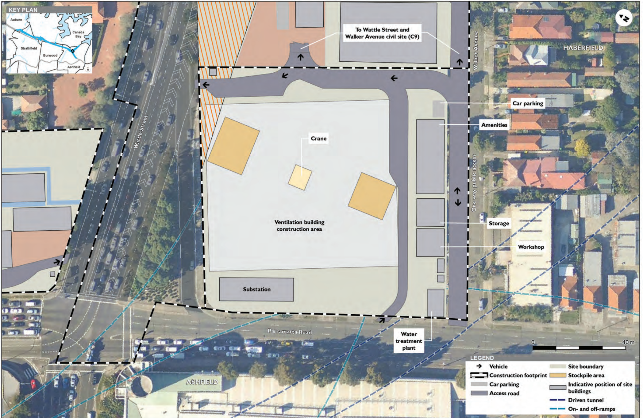
Figure 6.16 Indicative eastern ventilation facility layout (C8)
